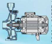
The lantern bracket design prevents contact with the pumps rotating parts, providing protection to the end user whilst allowing for inspection of the mechanical seal.
